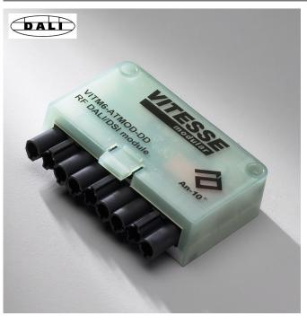
The VITM6-ATMOD-DD is a wireless controller with two output channels capable of controlling incandescent, fluorescent and compact fluorescent lighting when connected to Vitesse Modular Dimming Modules (refer to the user guide for the VITM6-S and VITM6-E for installation and wiring).
